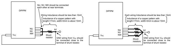
Low inductance shunt resistor like surface mounted (SMD) type is recommended.
