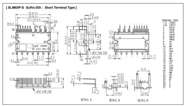
Note: Connect only one V<sub>NC</sub> terminal (No.12 or 19) to the system GND and leave another one open.
