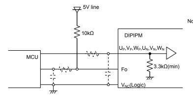
Note: The RC coupling (parts shown in the dotted line) at each input depends on user's PWM control strategy and the wiring impedance of the printed circuit board. The DIPIPM signal input section integrates a  $3.3 k\Omega(\text{min})$  pull-down resistor. Therefore, when using an external filtering resistor, please pay attention to the signal voltage drop at input terminal.
